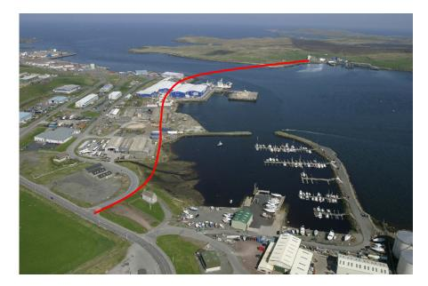
• **Option 2: High Level Bridge**: This option covers a high level bridge with an airdraft of 60m above MHWS over a 260m wide channel. The bridge would also be provided with wind shielding. It would allow two directional traffic and would have a 2m combined footway/cycleway on one side and a 0.6m wide verge on the other.
